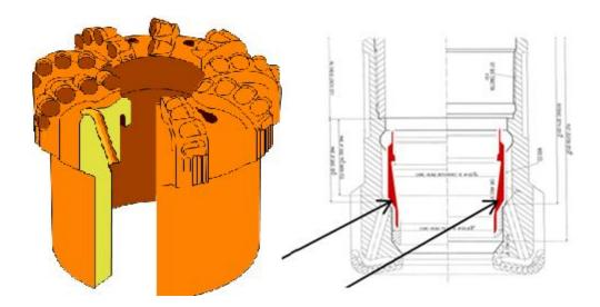
The internal geometry is determined by the ratio of the outer dimensions of the Lower Half of the Shoe and the inner dimensions of the core head.
