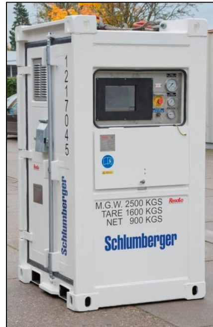
Formation Isolation Valve (FIV) charging unit type FIV-10.000/E fully automated
